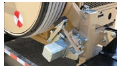
Hydraulic clamp allows for convenient safe reel change.
