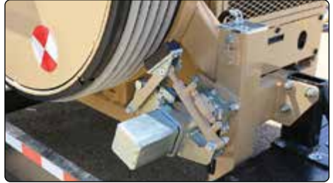
Hydraulic clamp allows for convenient safe reel change.
